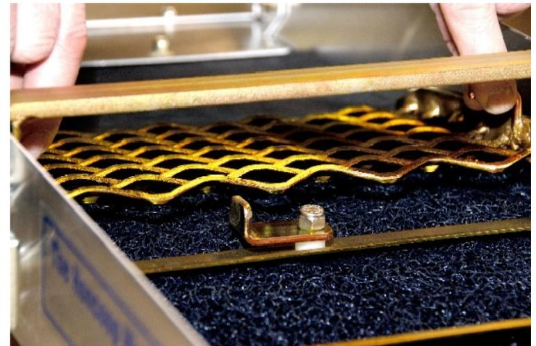
Pull up on the two tabs to remove the expanded metal.
