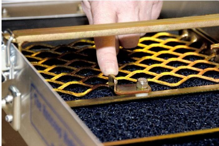
Swing the expanded metal hold-down lever left or right to start a quick cleanup. The latches do not have to be released on the main tray for the quick cleanup.
