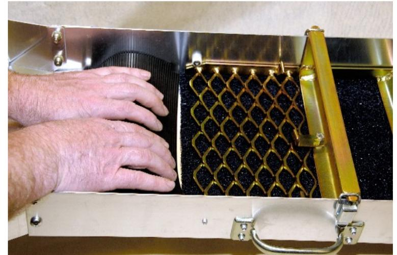
To reassemble, set the Mat, moss, and expanded metal back into the sluice first. Then, finish with the front Black Ribbed Mat by bowing it up to fit the rubber mat on top of the Moss, but under the expanded metal.
